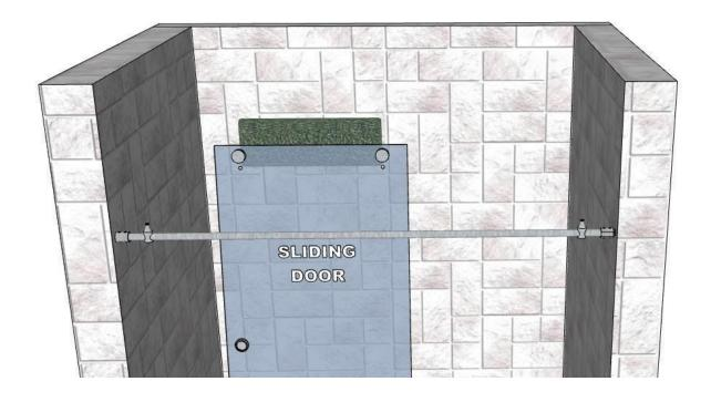
10. To attach the bar to the walls, slide both collars over their pucks. Tighten the screws to hold the collars in place, which in turn locks the roller support bar into position.
