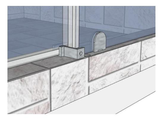
At the top, the PVC should be cut so that it stops  $\frac{1}{2}$ " below the anti-lift fitting of the sliding door.
