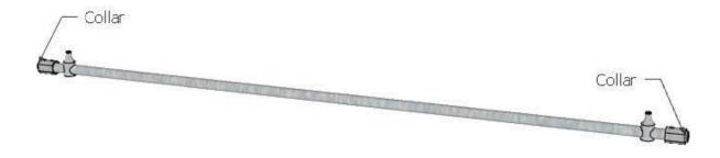
9. Hold the roller support bar, with its attached door stops and collars, so that the ends are flush with the pucks on both sides. Check to ensure that the bar is level - if it's not, then adjust the location of one or both pucks.
