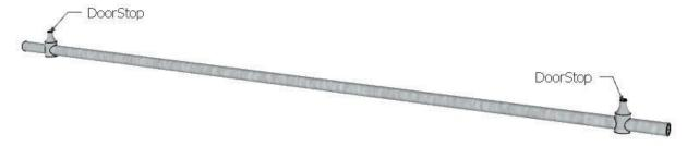
8. Slide both collars from the wall mount brackets onto both ends of the roller support bar. Use painter's tape here as well, to temporarily hold the collars in place.
